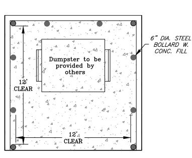
Typical Dumpster Enclosure – Plan N.T.S.
